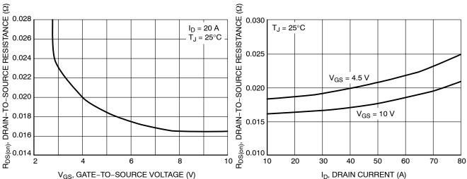
Figure 3. On-Resistance vs. Gate Voltage
