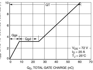
Figure 8. Gate-to-Source Voltage vs. Total Charge
