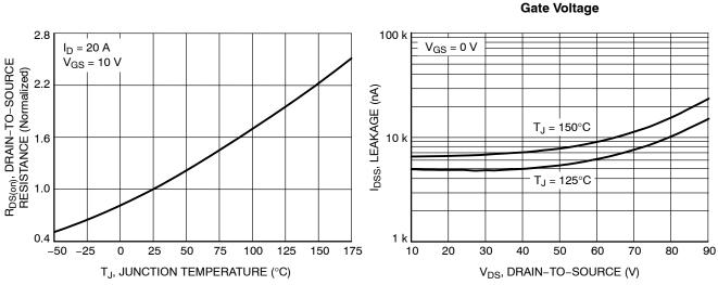
Figure 5. On–Resistance Variation with Temperature
