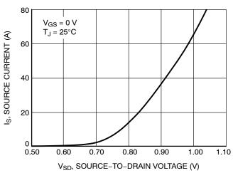
Figure 10. Diode Forward Voltage vs. Current
