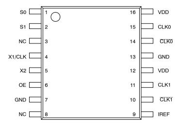
Figure 2. Pin Configuration (Top View)
