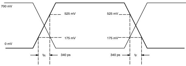
Figure 5. HCSL Output Parameter Characteristics
