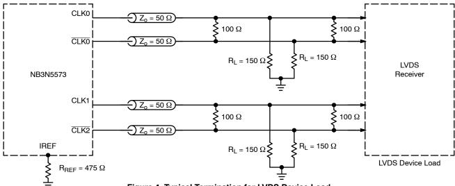
Figure 4. Typical Termination for LVDS Device Load
