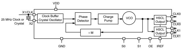
Figure 1. NB3N5573 Simplified Logic Diagram
