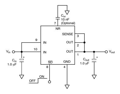
Figure 1. Typical Fixed Version Application Schematic
