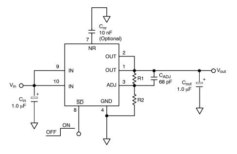
Figure 2. Typical Adjustable Version Application Schematic
