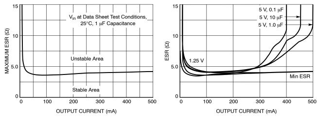
Figure 26. Stability with ESR vs.  $I_{out}$
