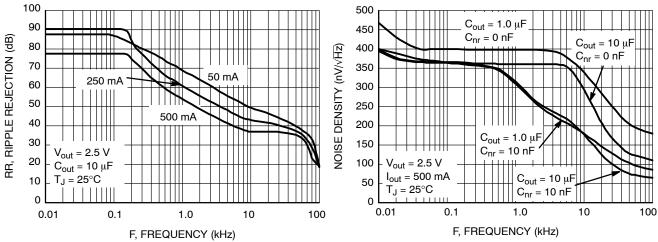
Figure 23. Ripple Rejection vs. Frequency
