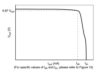
Figure 16. Output Voltage vs. Output Current
