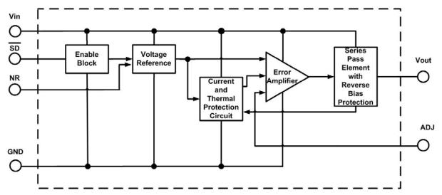
Figure 4. Block Diagram, Adjustable Output Version
