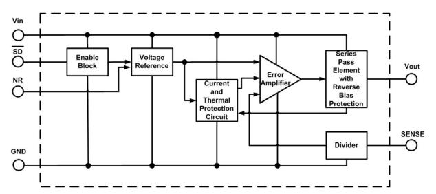
Figure 3. Block Diagram, Fixed Output Version
