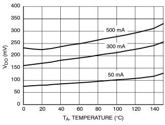
Figure 11. Dropout Voltage vs. Temperature 2.8 V Version
