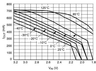
Figure 22. Output Current Capability for the 1.5 V Version
