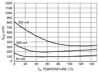
Figure 13. Dropout Voltage vs. Temperature 1.8 V Version
