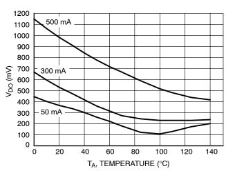
Figure 14. Dropout Voltage vs. Temperature 1.5 V Version
