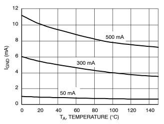
Figure 17. Ground Current vs. Temperature
